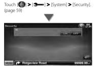
[SI] Turns the SI function on or off. If turned "ON", the security indicator on the front panel flashes when the vehicle ignition is off. ( P "ON")
